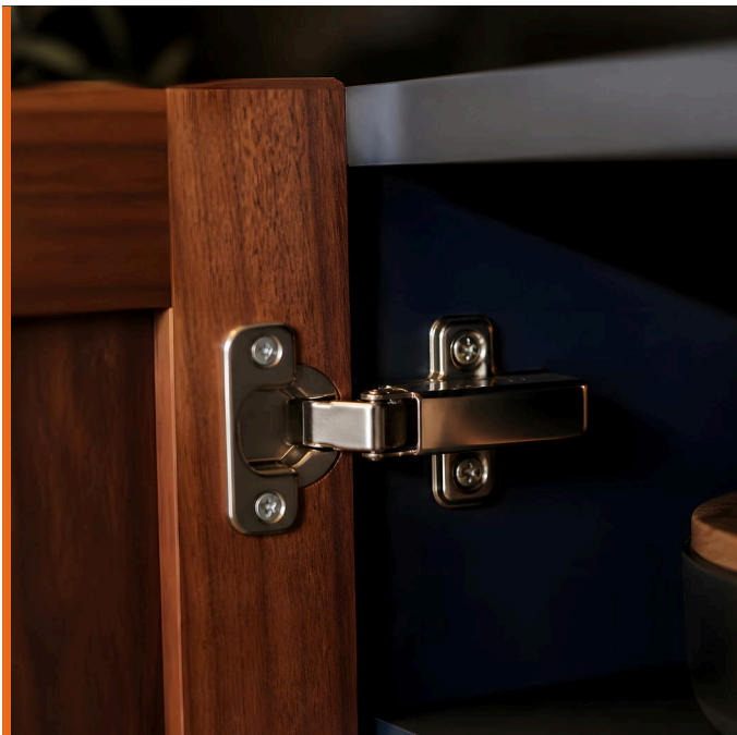
Clip-on arm on the mounting plate: snaps on by hand, releases with the button
