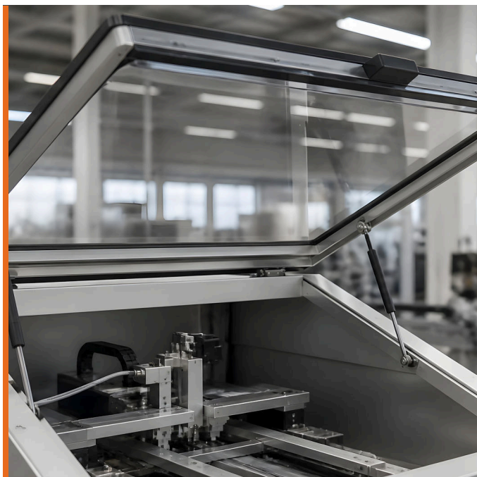
Machine guard: hinged cover on eyelet fittings, free articulation at both ends
