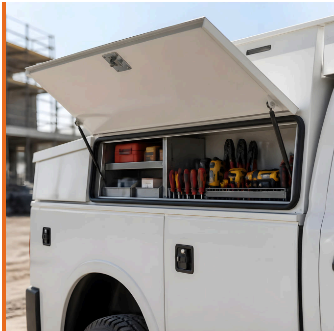
Work truck service body: upper compartment door held open on two springs
