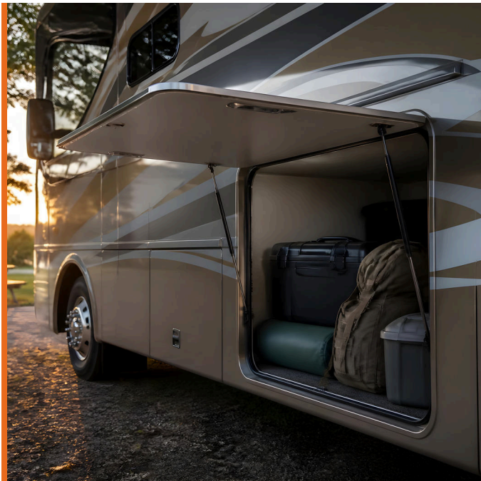
RV exterior storage bay: lift-up door that stays open while loading
