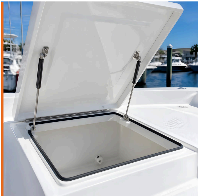
Boat deck hatch: a spring each side, mounted between lid and frame
