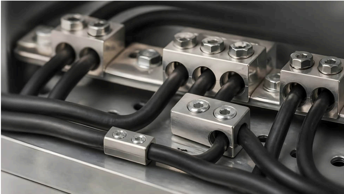
Panelboard connectors and a splicer-reducer in the gutter: multi-barrel bodies land parallel feeders on one bolt, the splicer joins two sizes in line.
