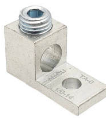
CT-T1H1-1-0A 1-Conductor 1-Hole Dual-Rated AL/CU 14 AWG-1/0 AWG 1/4in Stud
