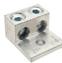
CT-T2H1-2-0A 2-Conductor 1-Hole Dual-Rated AL/CU (2) 14 AWG-2/0 AWG 1/4in Stud
