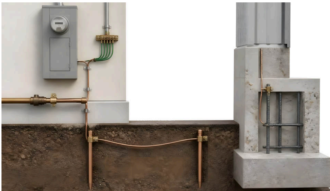
A complete grounding electrode system: rod electrodes with listed clamps, the water pipe bond within 5 ft of entry, the concrete-encased electrode, the intersystem bonding termination.
