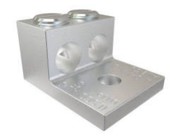
CT-T2H1-1-0A 2-Conductor 1-Hole Dual-Rated AL/CU (2) 14 AWG-1/0 AWG 1/4in Stud
